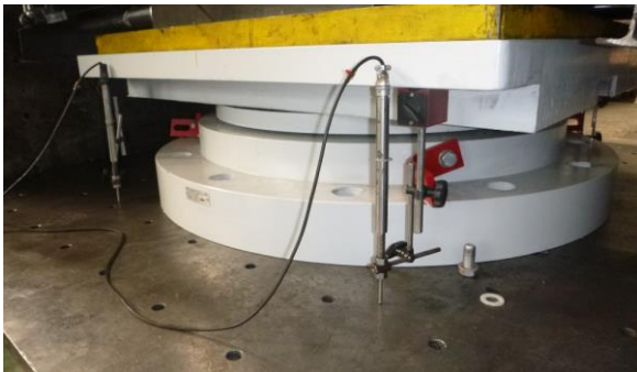
TETRON® CD guided sliding bearing test at ISOLAB testing facility Bridge at the Intersection of Prince Turki Rd. with King Abdullah Rd. (Saudi Arabia)
